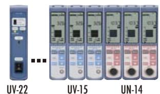
Configure a measurement system for up to 16 channels by linking the Sound Level Meter Unit UN-14 and Vibration Level Meter Unit UV-15. Each unit has its own display showing settings, measurement values, and a bar graph indication. Adding the Interface Unit UV-22 allows connection to a computer for control of settings and operation and transfer of measurement data.
